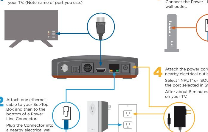
Attach second ethernet cable to a LAN port on your modem or router, and then to the second Power Line Connector.
