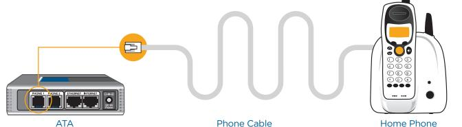
Using one of the Ethernet cables provided, connect one of the available modem LAN ports to the blue INTERNET port of the Analog Telephone Adapter (ATA).
